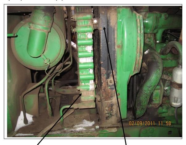
Condenser locates similar to factory style AC condenser. (shown) Fittings at the bottom.
