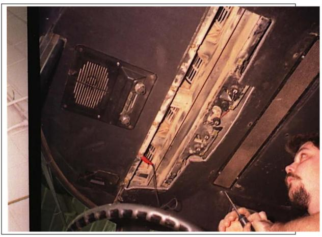
Temporarily remove the factory hydraulic cooler to install condenser.
